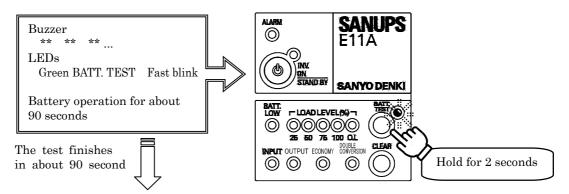
Check the green BATT. TEST indicator for the results of the test.
